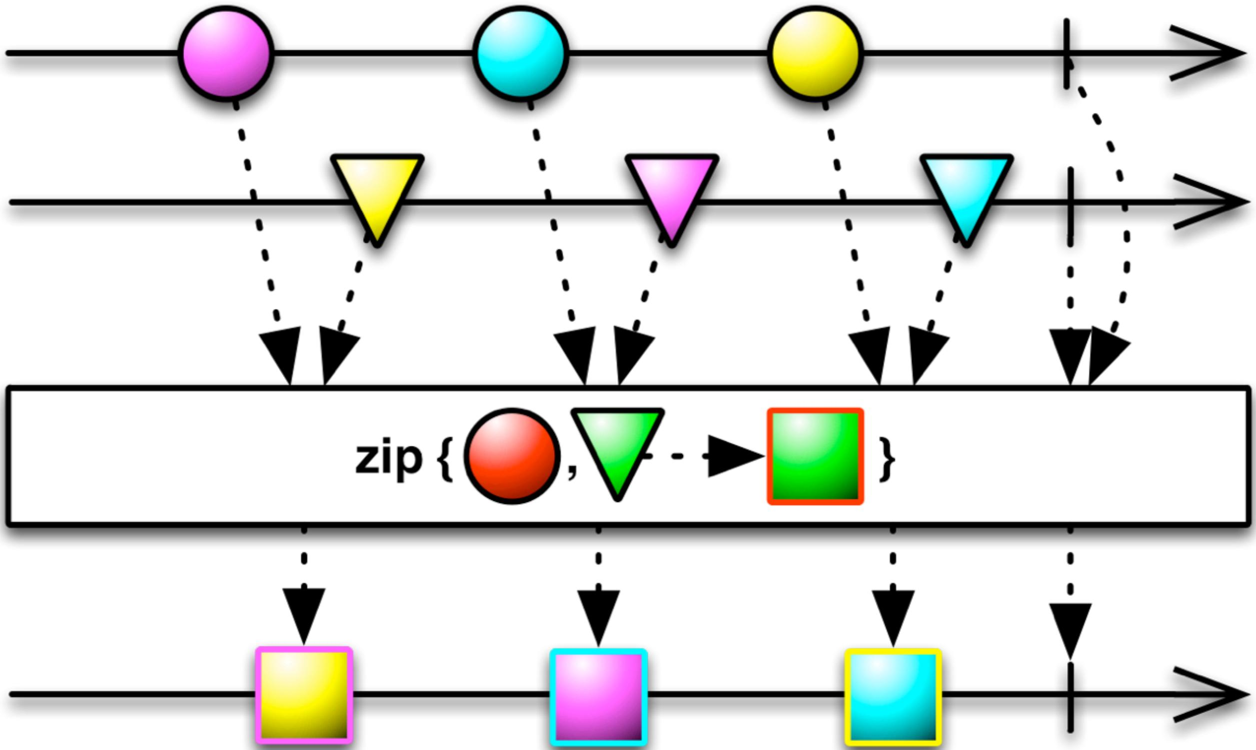
The 'zip' operator is used to combine Observable sequences of different types.
