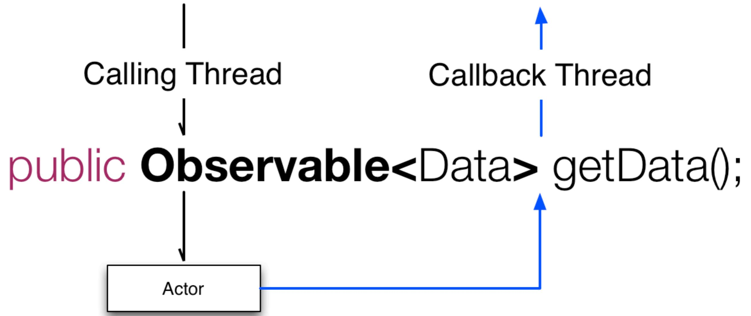
Do work asynchronously on an actor
