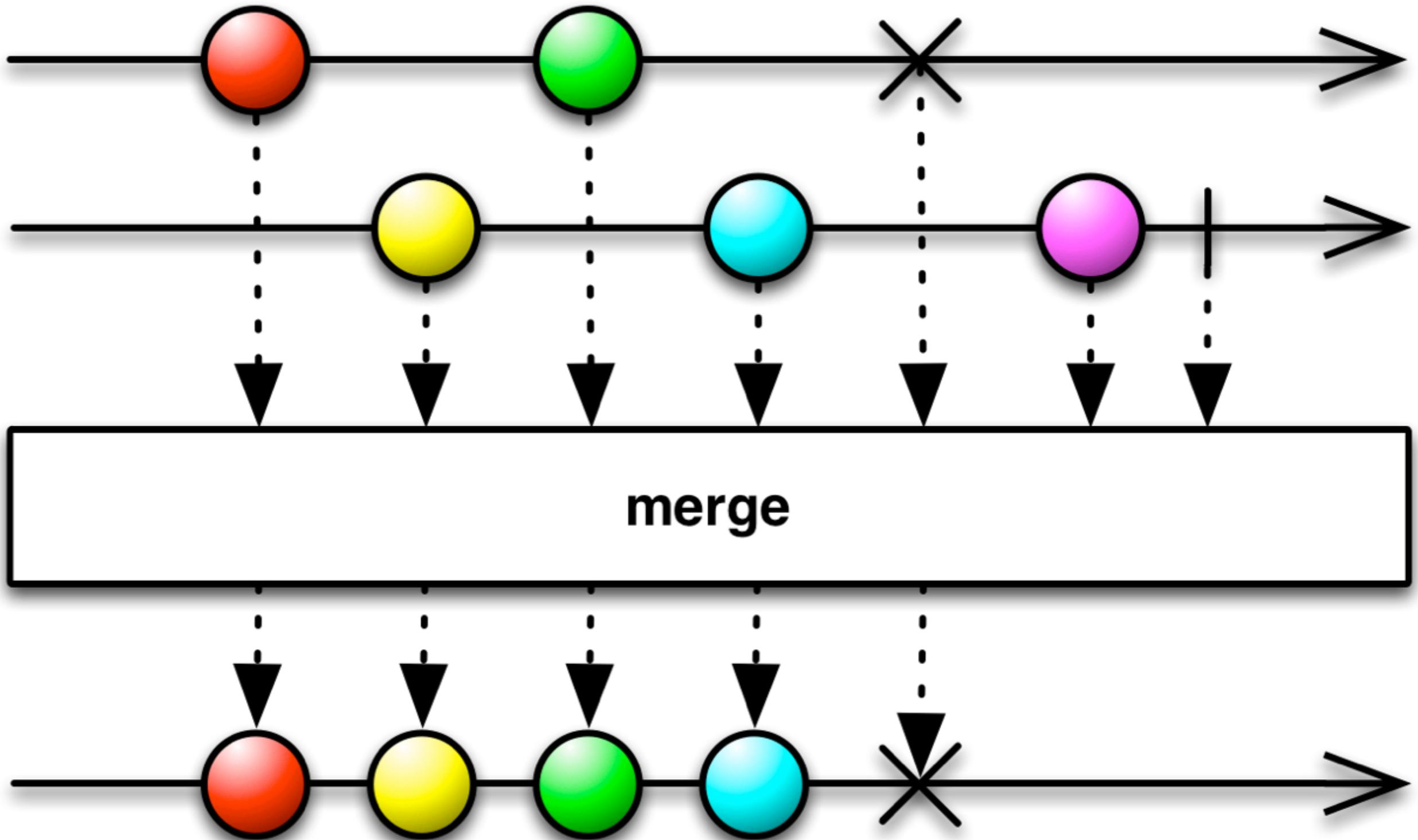
The 'merge' operator is used to combine multiple Observable sequences of the same type into a single Observable sequence with all data.
