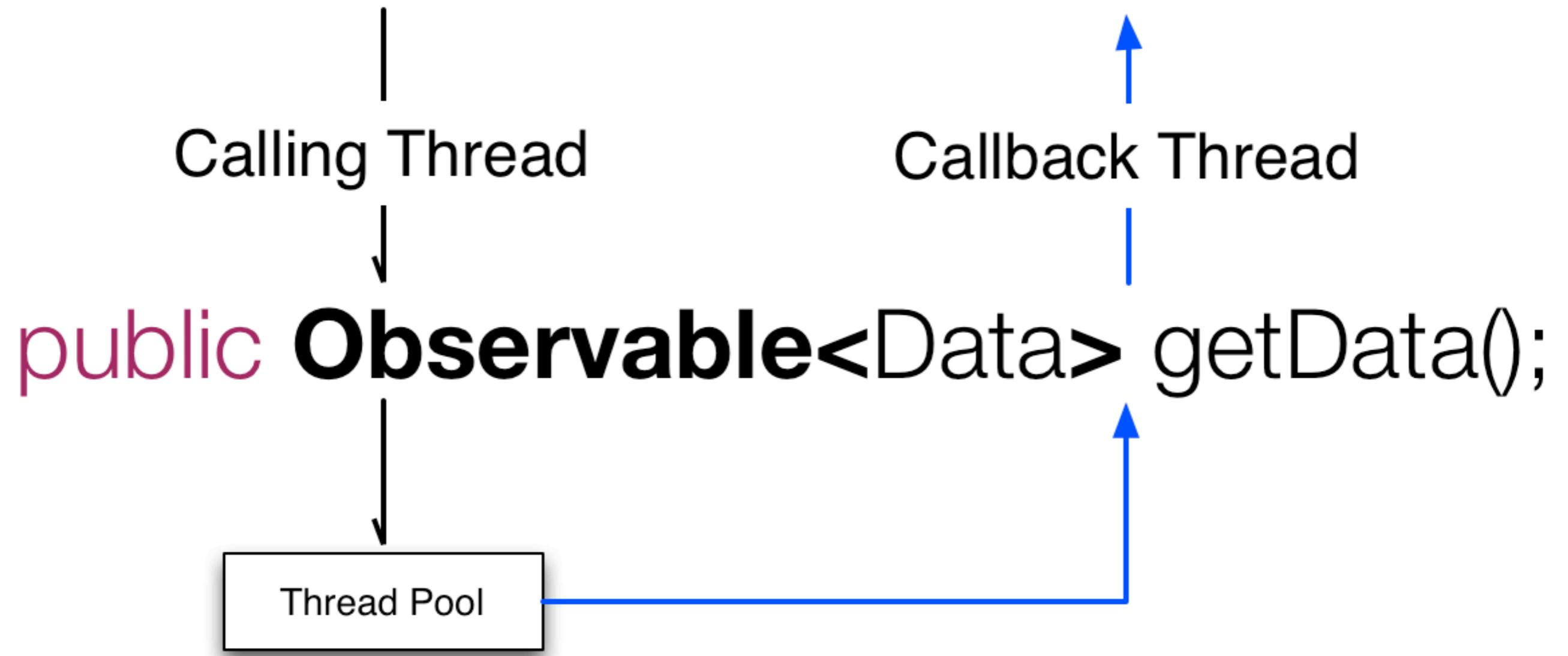
Do work asynchronously on a separate thread.
