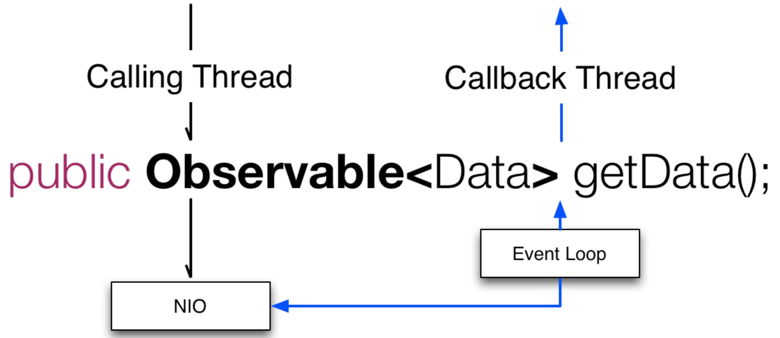
Do network access asynchronously using NIO
