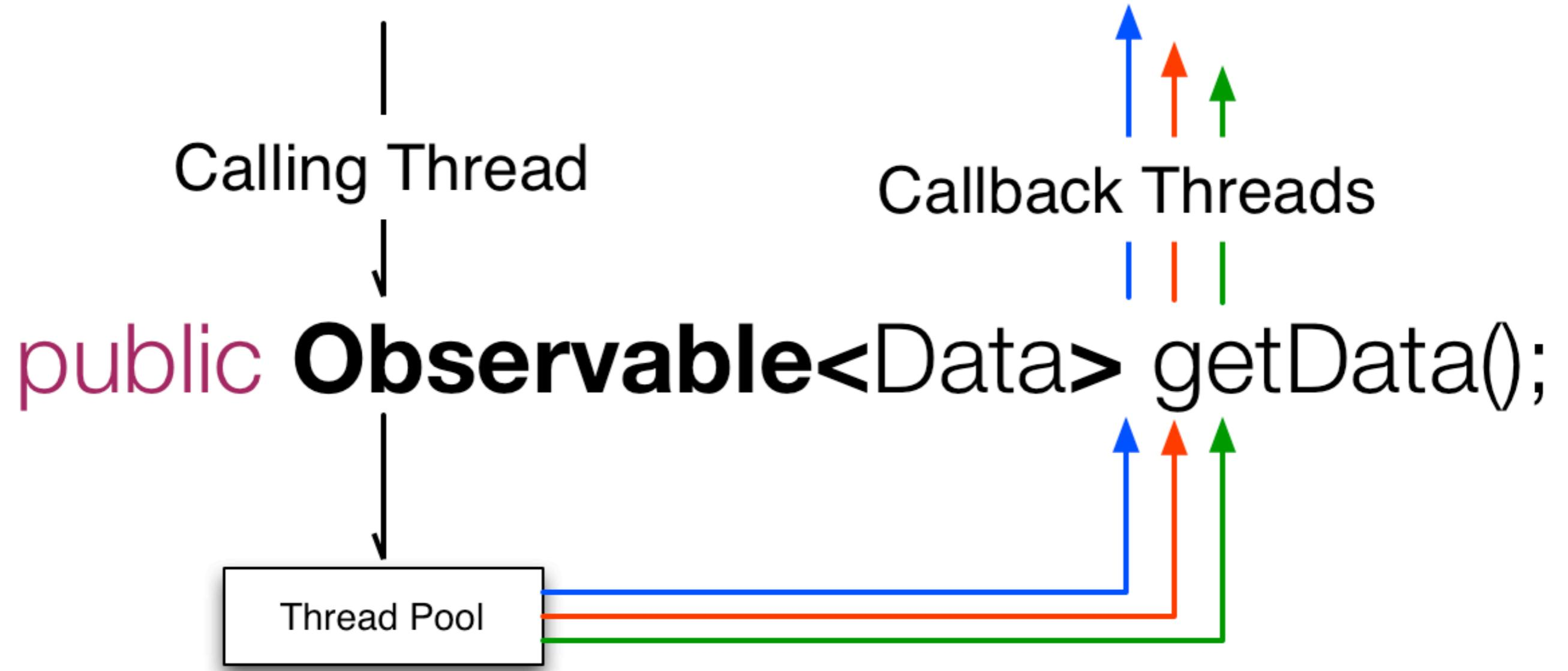
Do work asynchronously on a multiple threads.
