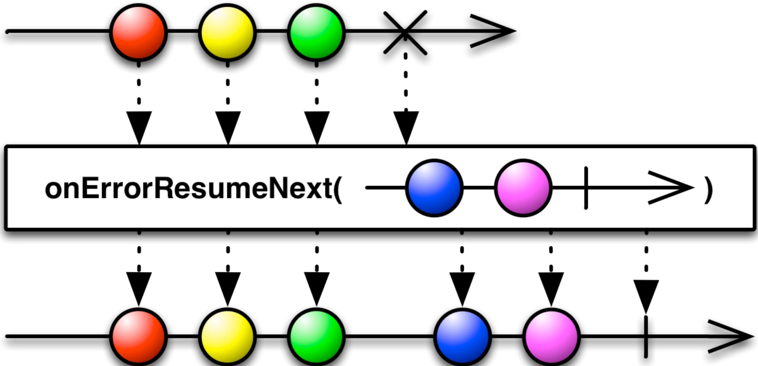
The 'onErrorResumeNext' operator allows intercepting an 'onError' and providing a new Observable to continue with.
