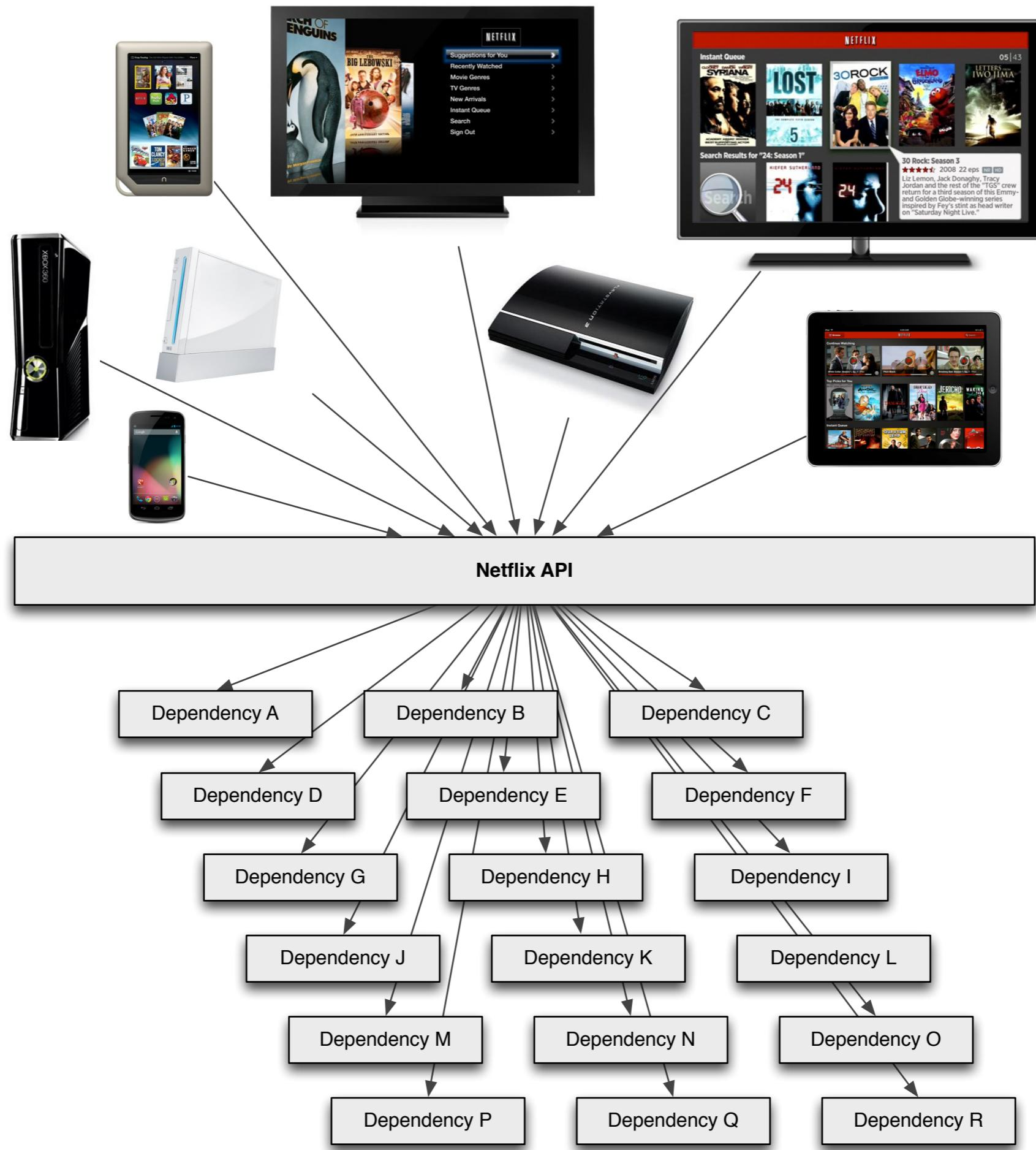
The Netflix API serves all streaming devices and acts as the broker between backend Netflix systems and the user interfaces running on the 800+ devices that support Netflix streaming.
