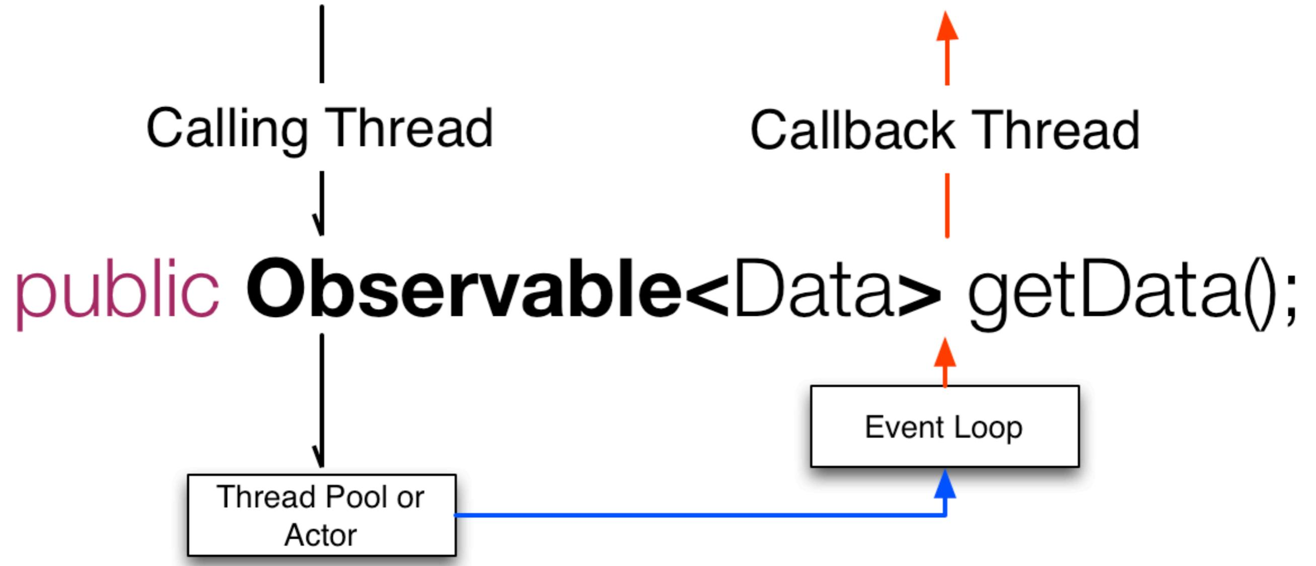
Do work asynchronously and perform callback via a single or multi-threaded event loop.
